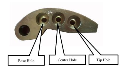
Remove the primary clutch and install the weights and primary spring. Remove secondary clutch and install new helix in proper setting, with spring. Inspect all internal clutch components for wear. If excesses wear is prevalent replace needed items.
