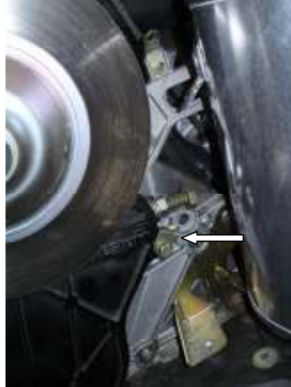
New spring clip installed under bolt
