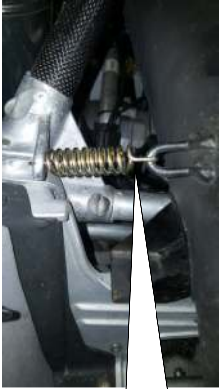
Be sure to always check spring tension to ensure proper sealing of pipe.
