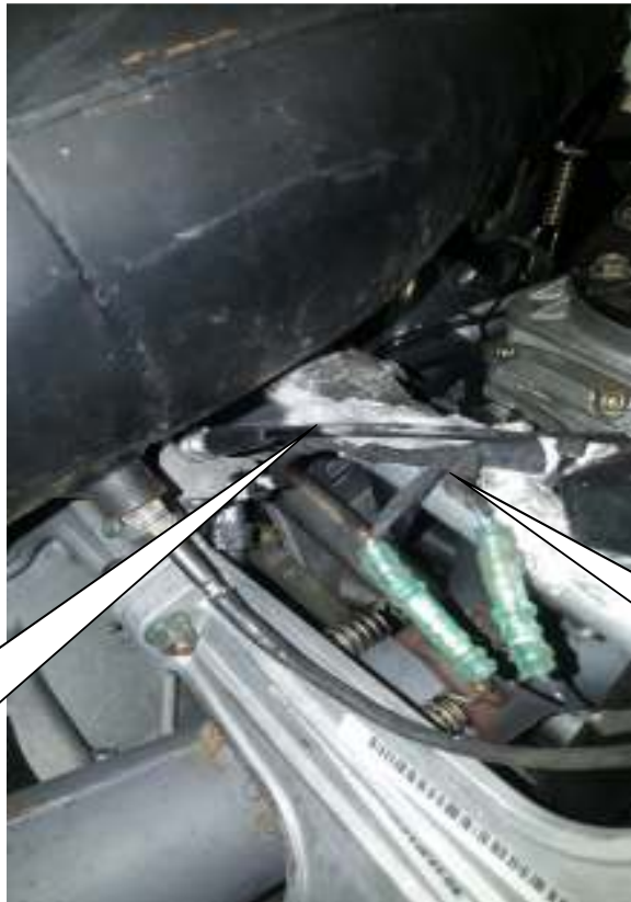
Zip tie cable down loosely, then cover with supplied heat tape
