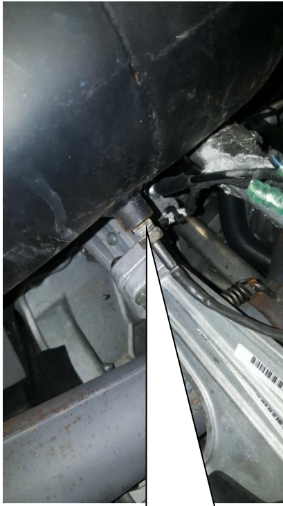
Stock Pipe sensor to be re-installed into Straightline Performance pipe.
