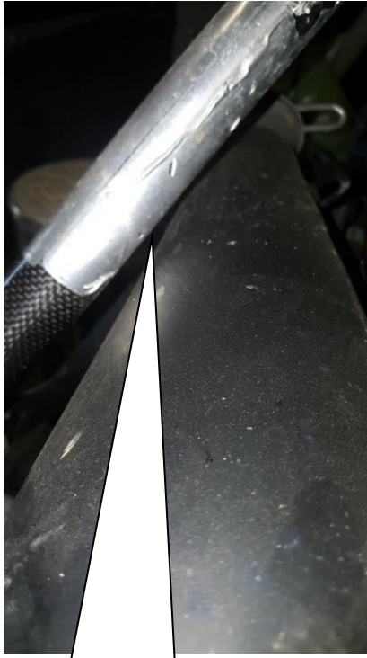
Be sure pipe has enough room to clear chassis components. Typically a 1/4" will suffice.
