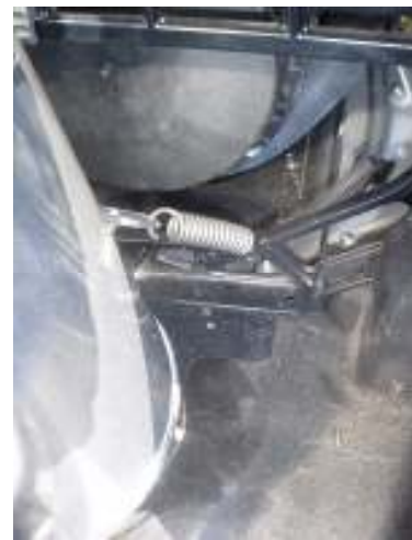
Front Lower Spring Installed #3
