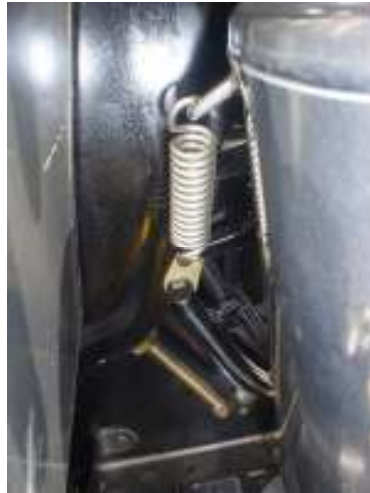
Rear Spring and Mount Added #2
