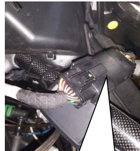
Unclip the main harness plug
