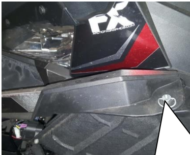
Unscrew these hood pins from both sides.
