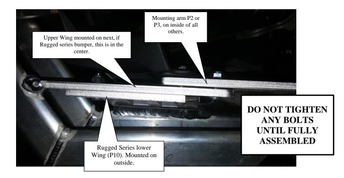
8. <u>Skid plate install:</u> flip machine on its side or elevate on a lift stand to gain access to rear holes on the skid plate. Drill Bottom holes (¼" drill bit) to fit Straightline supplied hardware and mount lower skid plate. Removal of the exhaust pipe is recommended if it has not been done already.
