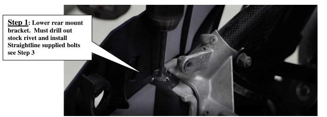
Install the two Bumper Arms (P2 & P3) hardware needed (P5 Qty 2, P6 Qty2, P7 Qty 4) The picture below shows the mounting locations on the rear. The upper support uses the stock location. 2019+ models are different than 2015-18 see pictures below
