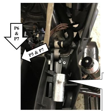
Notch cut outs designed for the stock belt holder to be re-installed onto the Straightline bracket. Use the stock plug wrench to support the holder.
