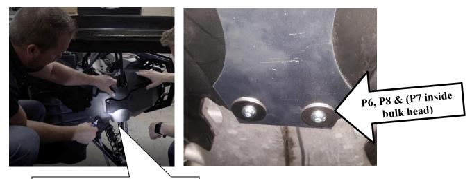
Drill Bottom holes to Straightline supplied hardware and mount lower skid plate. Removal of the exhaust may be required.
