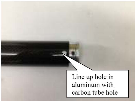
Line-up the holes before complete installation #1
