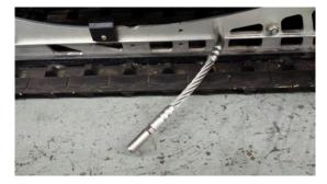
2. Test fit the Scratcher cable, 9/16" mounting bolt, and mounting bolt washer on the rail, and position as desired (elbow angle should be no more than 45 degrees back to insure adequate surface pressure).
