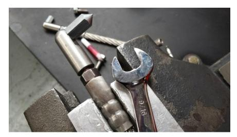
7. Tighten the 9/16" jam nut to 25ft pounds against the base of the scratcher cable, not the base of the head.
