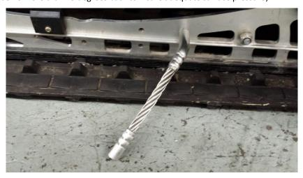
3. Install threaded head (with scratcher carbide tip installed) into scratcher cable. Place several drops of red Loctite on the threads closest to the scratcher cable.
