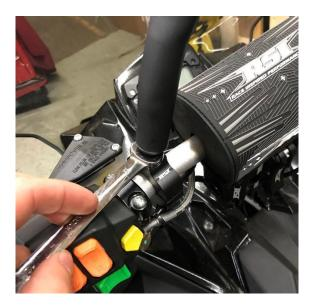
Step 5: Align grab bar and tighten bottom caps of grab bar mounts using 4 mm Allen wrench
