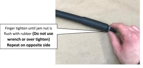
**Step 2:** Install grab bar into Grab Bar mounts spin on until bottomed out and minimal thread is exposed.
