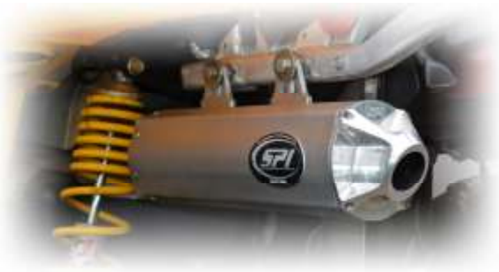
New SPI Muffler installed
