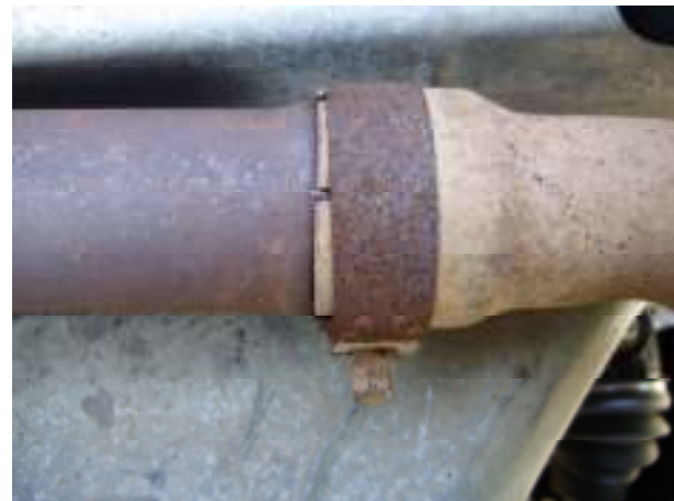
Unbolt clamps and slip on SPI muffler Re-clamp with SPI supplied clamp
