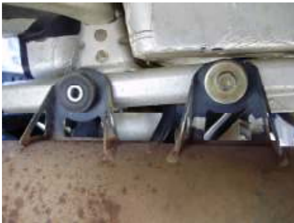
Remove both stock bolts and muffler. Re-use the stock bolts to install SPI muffler
