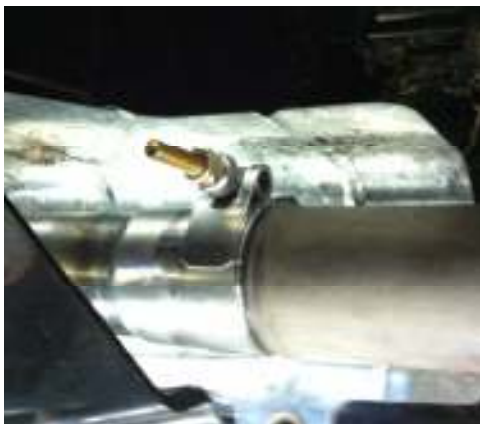
New SPI Clamp Installed
