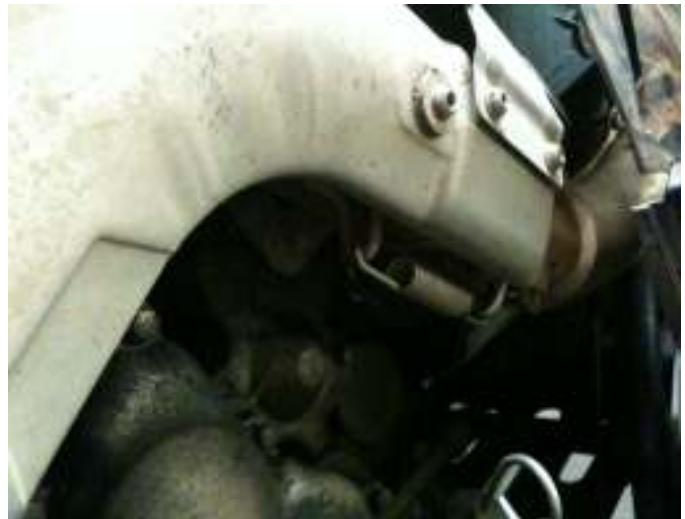
Unspring the 2 springs that attach the stock muffler to the header pipe
