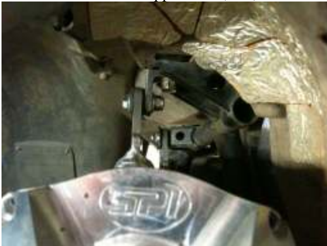
Install the L bracket under the rear rack bolt as shown in the above picture
