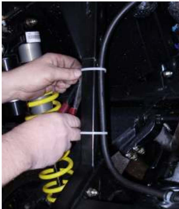
Use the supplied zip ties to tie off hose and wires on drivers side frame next to the shock.
