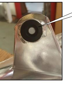
Install stock grommet into new Straightline
