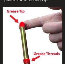
3. Install puller, hold primary clutch with primary holder and tighten until primary clutch pops off.
