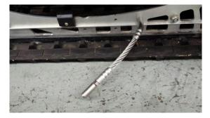
2. Test fit the Scratcher cable, 9/16" mounting bolt, and mounting bolt washer on the rail, and position as desired (elbow angle should be no more than 45 degrees back to insure adequate surface pressure).
