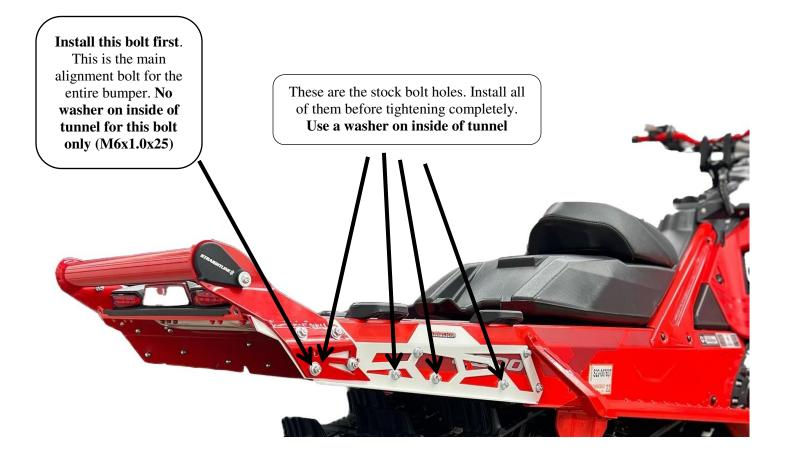
Drill these holes after all the stock bolts are installed and tight. Drill using a 6mm (1/4") drill bit. (Install and tighten bolts using washer on inside of tunnel)
