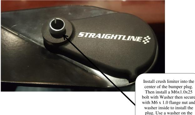
center of the bumper plug. Then install a M6x1.0x25 bolt with Washer then secure with M6 x 1.0 flange nut and washer inside to install the plug. Use a washer on the outside only, no washer on the inside.
