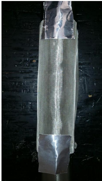
Stainless Wrap with heat tape to hold
