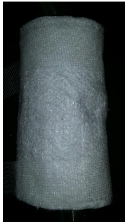
Wrap the packing and hold with white tape.
