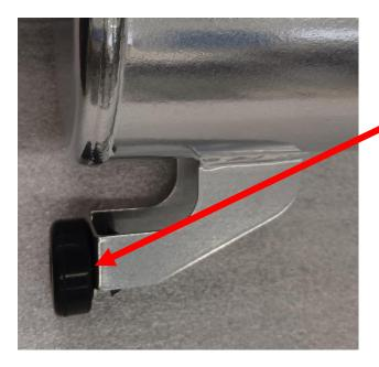
Install the stock muffler grommet as shown here. The wider part must be on the bottom. You can add a small amount of grease to ensure the grommets slide into the muffler and pins to be fully seated.
