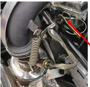
Your stock muffler used 2 hitch pin clips and 2 large washers on the 2 upper mounting pins. The Straightline muffler only has 1 pin. Be sure to install the other clip and washers into place even though there is no mount there. This way the clip is completely installed and will not fall.
