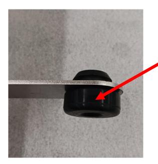
Install the stock muffler grommet as shown here. The wider part must be on the bottom. You can add a small amount of grease to ensure the grommets slide into the muffler and pins to be fully seated.
